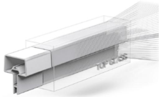
**Pullwinding** is used for producing tubular profiles with high transversal rigidity and mechanical resistance. This production process differs from pultrusion with respect to way the fibreglass is positioned for reinforcing the profile. In order to obtain superior rigidity pullwinding uses both roving placed longitudinally and circumferentially with respect to the profile's axis.
