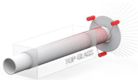
**Centrifugal casting** is used to make fiberglass composite poles in the shape of a truncated cone (GFRP tapered poles) with a maximum length up to 13.6 meters in one piece only, with a high degree of dimensional and physical-mechanical repeatability. It is mostly appreciated in lighting poles and supports for electricity, telephone and over-head lines.
